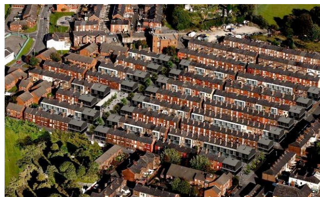
Toxteth Street from the air with visualised improvements by Mark Hines including new blocks at the ends of terraces and prefabricated rear extensions. Original photo: Jonathan Webb
